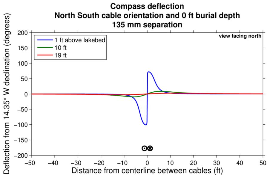
Figure 4. Compass deflection (degrees) from 14.35 degree W declination above north-south oriented cables on the lakebed, cables separated by 135 mm, and northward current in the eastern cable.
